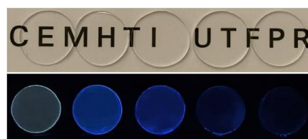
Fig. 1. Transparent CgCAF samples (top) and the same samples under UV light irradiation (bottom)
